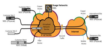
First is its ability to 'deploy anywhere'. This is based on a VNS 'site' being a collection of virtual functions that can be deployed in VMs anywhere and securely integrated with the other VNS nodes over IP Sec (or other encapsulations and links). 'Anywhere' in this case can be
